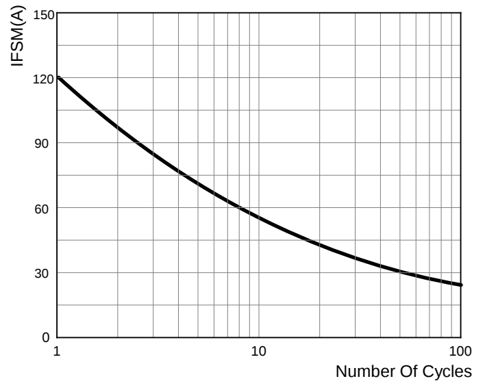
FIG 2: MAXIMUM NON-REPETITIVE FORWARD SURGE CURRENT
