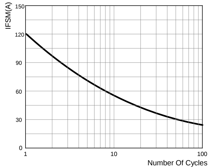
FIG 2: MAXIMUM NON-REPETITIVE FORWARD SURGE CURRENT
