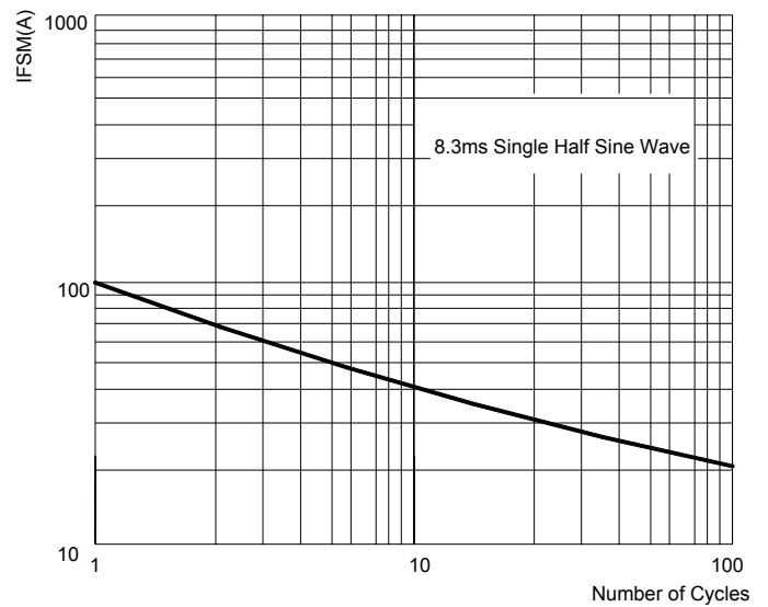
FIG.2: MAXIMUM NON-REPETITIVE FORWARD URGE CURRENT
