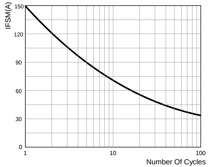
FIG 2: MAXIMUM NON-REPETITIVE FORWARD SURGE CURRENT
