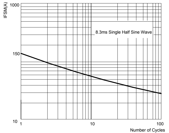
FIG.2: MAXIMUM NON-REPETITIVE FORWARD URGE CURRENT
